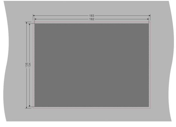
Cutout dimension: 183mm(W) \*135mm(H). Dashed box dimensions for the controller. The controller is fixed by 4 special fittings.
