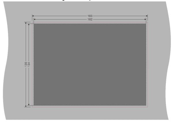
Cutout dimension: 183mm(W) \*135mm(H) . Dashed box dimensions for the controller. The controller is fixed by 4 special fittings  $_{\circ}$
