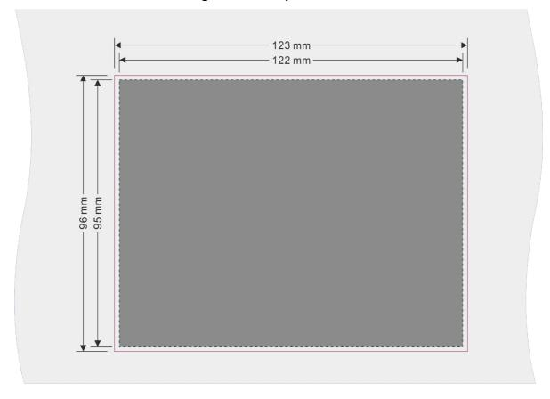
Cutout dimension: 123mm(W) x 96mm (H), Dashed box dimensions for the controller.
